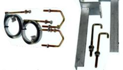
This Double Chimney bracket is ideal for use when a longer mast is required. It allows for greater spacing between mounting points. We recommend dropping a longer mast down below the lower bracket to balance the weight of the mast above the top bracket. Use with your existing pole or mate with one of our lightweight extendable masts such as our 3000mm to 3500mm mast. See our section on masting.
